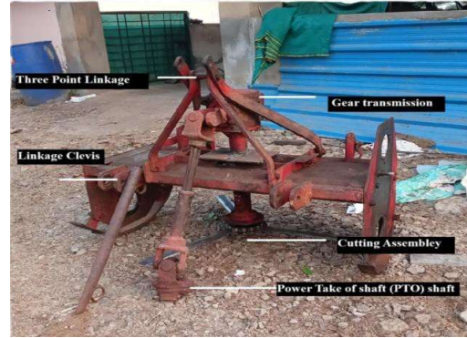
Fig. 1. Diagram of grass cutting flail mower (left) and block diagram of the proposed model (right).
