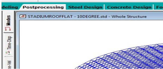
Fig 9 Mode Shape for Inclined Roof
