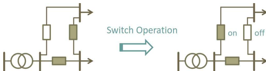
Figure 5. Basic concept of Reconfiguration of distribution network (RODN).
