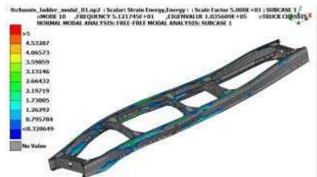
Figure 8-2 nd Order Torsion Analysis (51.22Hz)
