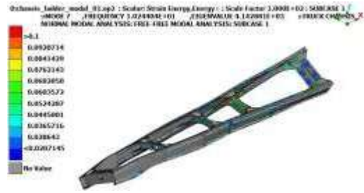
Figure 5-1 st Torsion Mode Analysis (10.24Hz)
