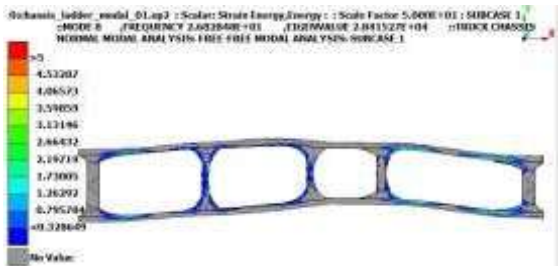
Figure 5-1 st Torsion Mode Analysis (10.24Hz)
