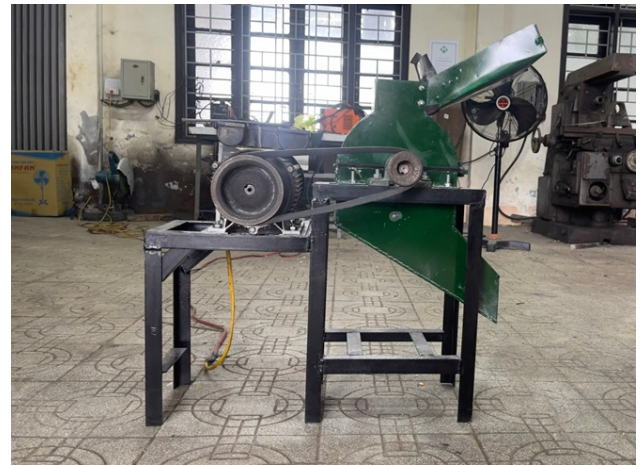
Figure 3. The final fabricated prototype of the corn hammer mill
